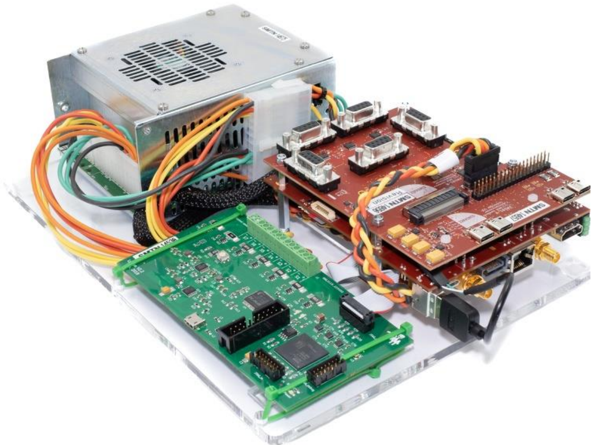
FIGURE 2 - TULIPP STARTER KIT WITH LYN SYN POWER MONITOR
